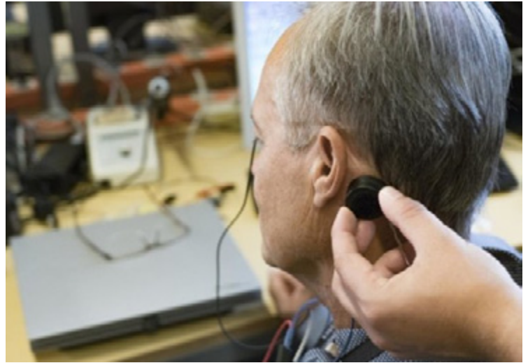
The vibrating device is small and compact in size, and optimised to provide an adequate sound level for triggering the reflex at frequencies as low as 250 Hz. Credit: Johan Bodell/Chalmers University of Technology
